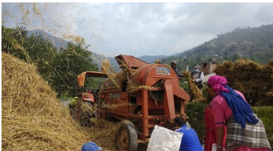
Photo 4: Tractor attached Thresher for Wheat harvesting
